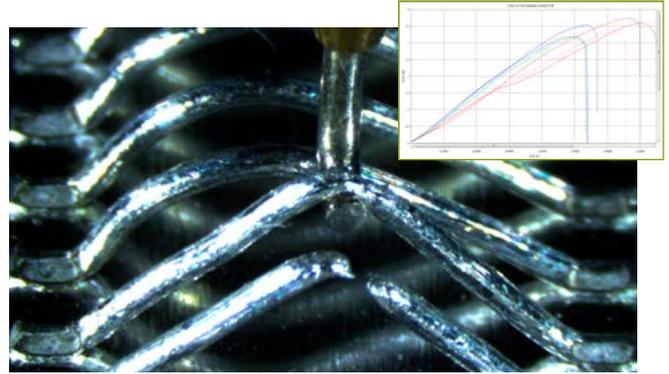
Heavy gauge wire 0.5mm diameter wire bonds prior to shear and pull testing, inset shows typical forces recorded.
