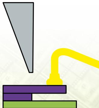
Figure 1. Alignment of shear tool with ball bond
