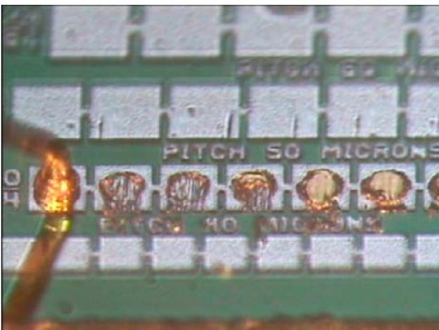
Figure 6. Typical view as seen through a Borescope with 330 micron FOV
