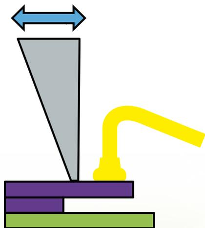
Figure 3. Shear tool being slowly raised until oscillating force is reduced to zero
