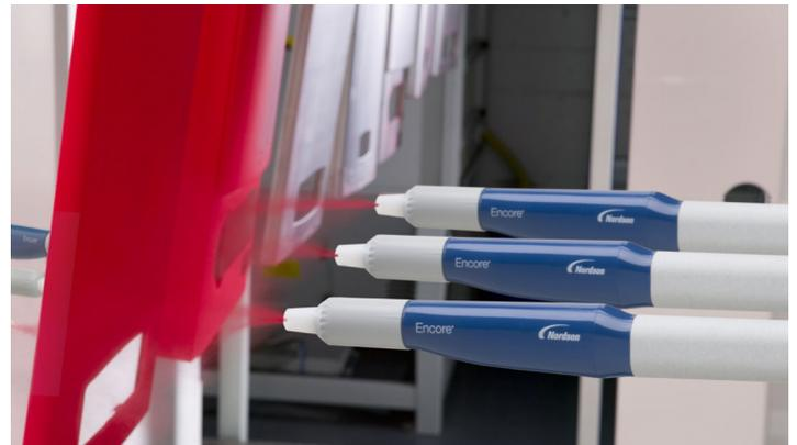
Encore HD guns are perfectly suited for use with the ColorMax® fast-color-change powder coating and recovery booth systems. Providing reclaim-to-reclaim color change in generally 5 to 10 minutes, the ColorMax system also ensures optimum application area air flow and control for maximum coating performance and efficiency in today’s lean manufacturing operations.
